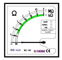
MEG-1000 is an electronic device that measures the insulating resistance between the ground and one phase of an insulated neutral network (IT).
